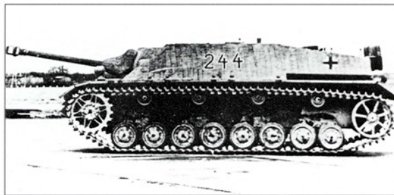
'Guderian's Duck' – the Jagdpanzer IV, armed with the 75mm Pak 39, 48 calibres long. Marking positions and styles are typical of this vehicle. Side skirts were normally carried; note also the Zimmerit finish. (RAC Tank Museum)
