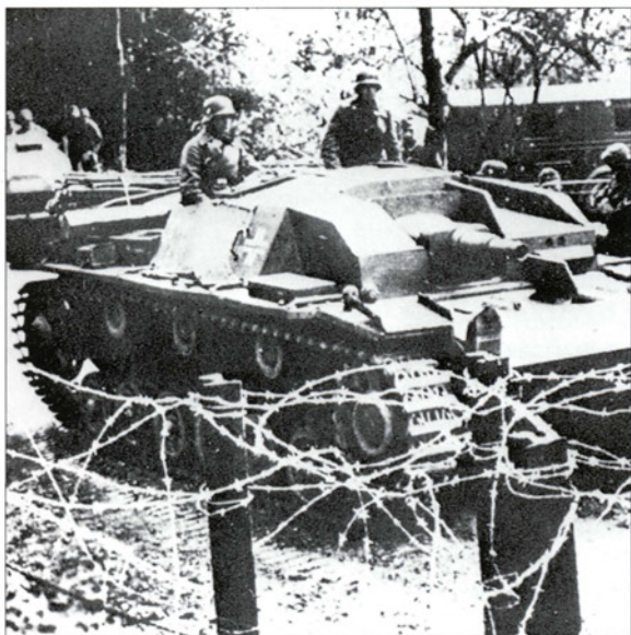
One of the two dozen or so StuG M assault guns to see service during the 1940 French campaign with Batteries 640, 659, 660 and 665. This is almost certainly an Ausf. B, employing the drive sprocket and idler of the narrow-tracked Ausf. A with spacer rings. The angled, spaced armour on the superstructure side is clearly visible, as is the broad V-shaped 'cut out' right of the gun, above the driver's compartment, leading back to the aperture of the gunner's sight. (RAC Tank Museum)
