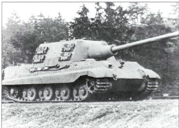
Weighing over 70 tons and mounting a 128mm gun, the Jagdtiger was the most powerful armoured fighting vehicle of the war. Its practical value was less striking however: it was subject to breakdowns and had a low rate of fire. (RAC Tank Museum)
