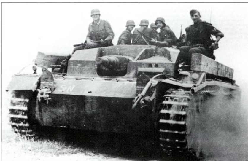
Another Ausf. B, photographed in the early stages of 'Barbarossa' with a load of infantry. The heavy 'unditching beams' are typical additions to the external stowage. The designation on the glacis suggests a battery HQ ('Stab') vehicle. (Bundesarchiv)
