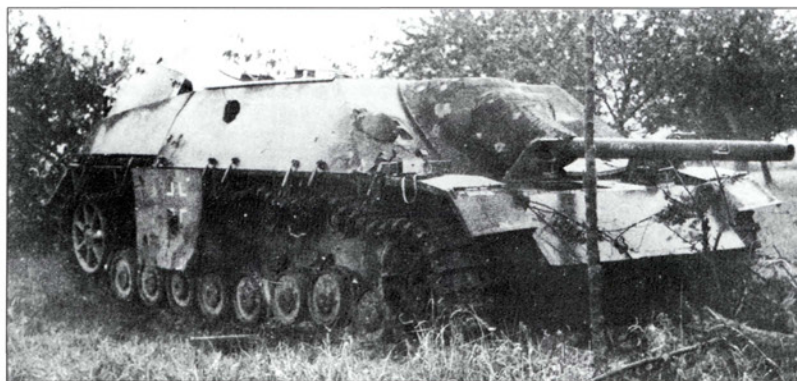
Later models of the Jagdpanzer IV mounted a 70-cal. gun without muzzle brake. This badly battered example fell to two well-placed flank shots in a Normandy orchard. To the left of the mantlet is the swivelling conical cover of the machine-gun port. At 6ft 1in, three inches lower even than the early model StuG III, this formidable tank destroyer could adopt concealed firing positions in the slightest fold of dead ground. (RAC Tank Museum)
