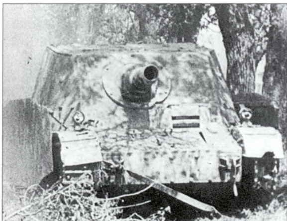
An abandoned Brummbär with skirt armour: note the late driver's vision block, identical to that used on the Tiger Ausf. E, and details of the ball-mounted 150mm howitzer.
