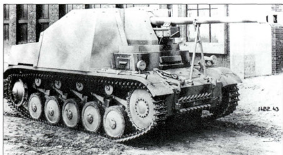
The Marder II mounted the 75mm Pak 40/2 anti-tank gun on the chassis of the PzKpfw II Ausf. A, B, C and F. (RAC Tank Museum)
