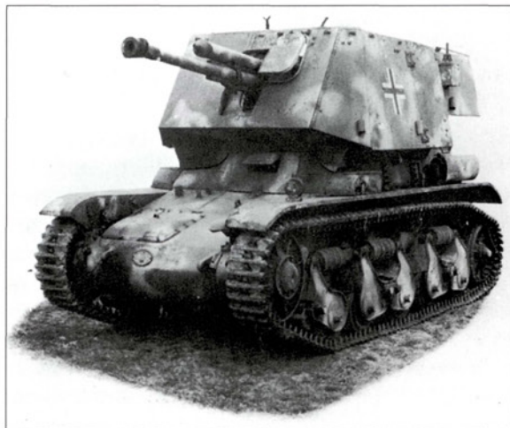
A number of obsolete French chassis were converted to the tank destroyer role. This vehicle mounts a 47mm anti-tank gun on the chassis of an R.35 tank: few were built, and those used mainly for training. (RAC Tank Museum)
